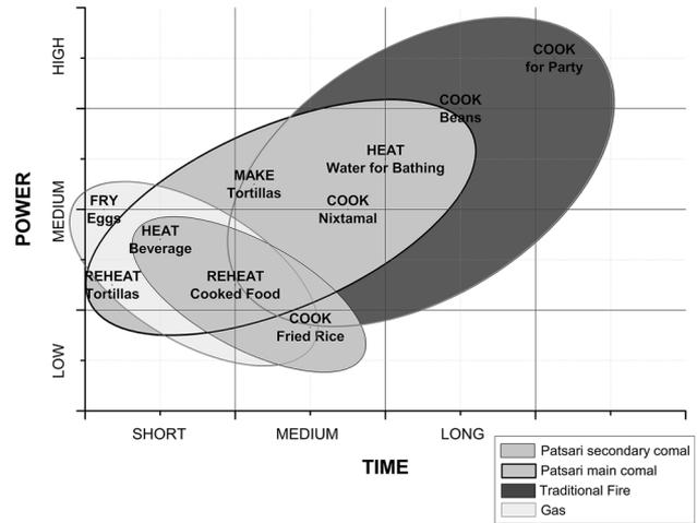
**Figure 8.** Definition of niches in the context of stove stacking for the case of the Patsari chimney stove, traditional open fires, and gas stoves in Central Mexico (estimated needs for a typical household size of 4–5 people).
