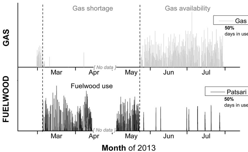
**Figure 5.** Seasonal stacking of a gas stove and a fuelwood Patsari stove seen during an LPG shortage, as measured by SUMs. The SUM traces represent fluctuations in stove temperature over time due to stove use. Both stoves have a long-term average of 50% day in use.
