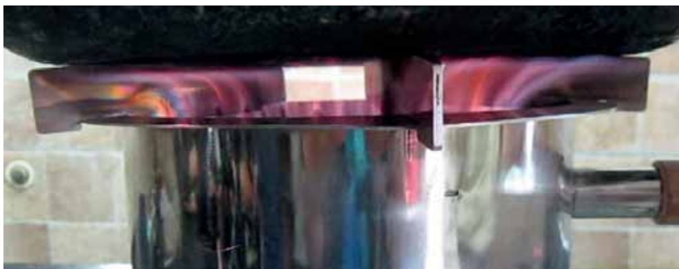
Photo 4.62 Clean flame of a 150 gasifier burning rice husk
