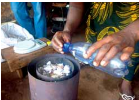
Photo 2.17 Metering kerosene with a bottle top before sprinkling it onto the fuel
