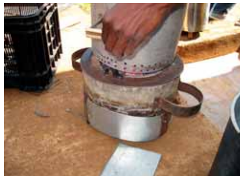
Photo 2.8 Lifting up the top part; no need to turn the hot stove over ...
