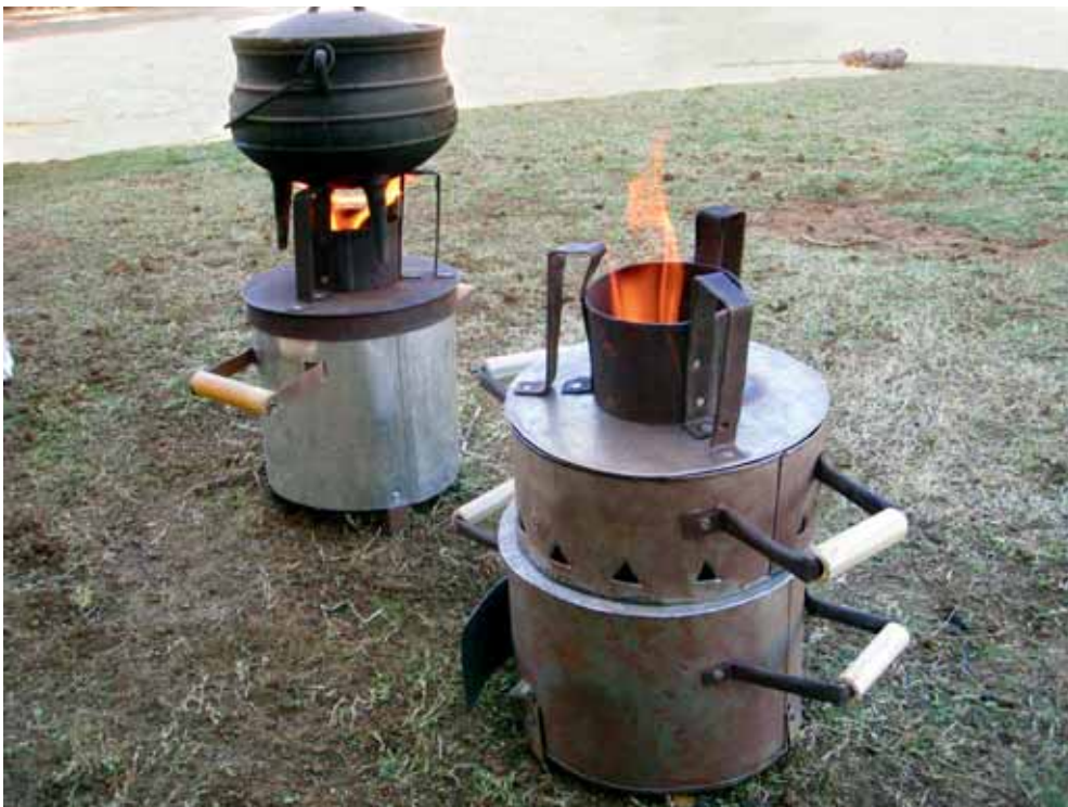
Photo 0.4 A PekoPe char-making gasifier (left) and a TChar stove that can burn char
