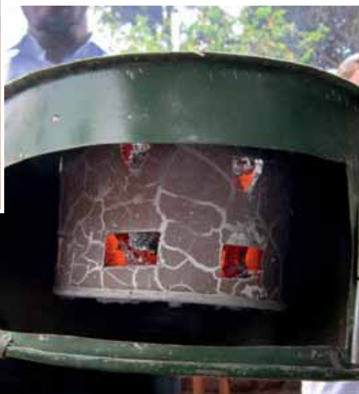
Photos 2.4 + 2.5 Char created from corn cobs in a gasifier can still be used to continue cooking
