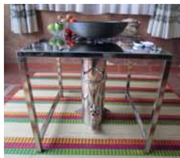
Photo 4.64 The 150 gasifier in a stainless-steel enclosure
