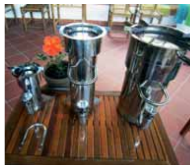
Photo 4.65 Left to right: The short reactor for pellets, the 150, and 250 gasifiers
