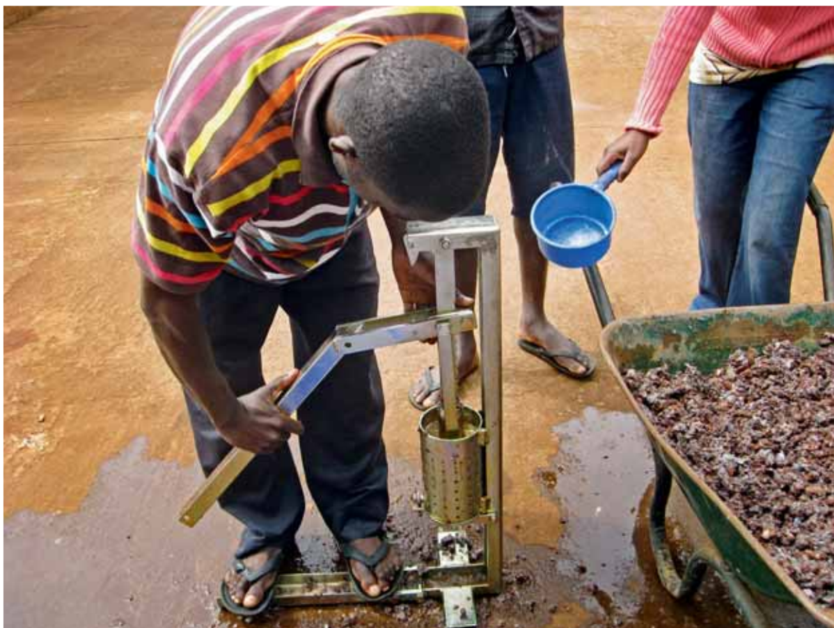
Photo 3.19 Ratchet press used in Malawi
