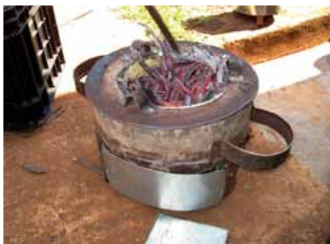
Photo 2.9 ... gravity allows the char from the bamboo to fall into the TChar-base
