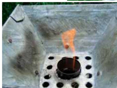
Photos 4.4 + 4.5 Everything-nice burners retrofitted in a charcoal stove from Benin
