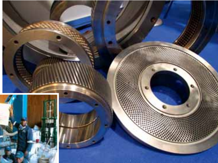
Photo 3.25 A flat die and rollers with radial grooves
