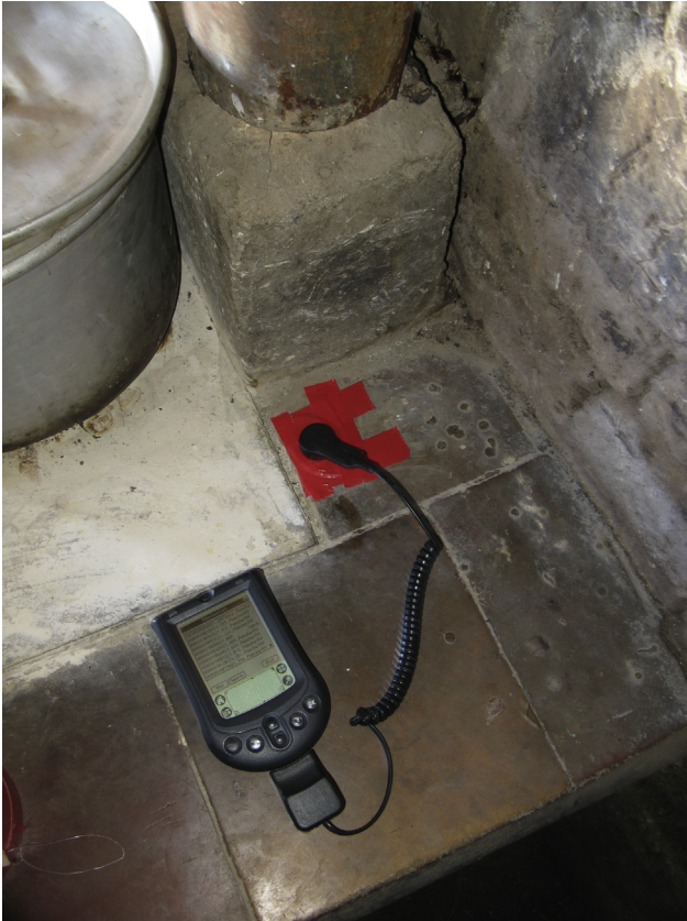
Fig. 1 – Small temperature dataloggers were used as Stove Use Monitors (SUMs). The SUMs, attached to the chimney-cookstove body, were programmed bi-monthly in the field and the data was downloaded using PDAs.
