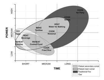
**Figure 8.** Definition of niches in the context of stove stacking for the case of the Patsari chimney stove, traditional open fires, and gas stoves in Central Mexico (estimated needs for a typical household size of 4–5 people).
