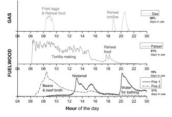
**Figure 7.** Stacking of gas stove, Patsari stove and two open fires used simultaneously on a typical day, measured with SUMs.
