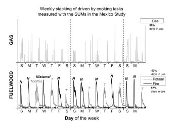
Figure 6. Stacking of multiple stoves and fuels on a weekly basis, measured with the SUMs. The gas stove is used daily to prepare meals and the Patsari stove and traditional fire are used on alternating days of the week for cooking tasks specific to making tortillas.
